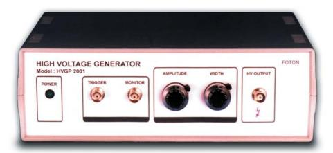
HVGP 2001 is a small and portable high voltage generator. It generates HV output pulses with regulated amplitude and temporal width. There are two modes of operation: single pulse mode and repetition mode. Auxiliar TTL output yields pulsewidth monitoring. High voltage output is galvanic insulated and leads into centres of two BNC sockets.
