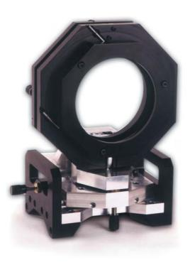
OMS 120 is an optical mount for non-standard optical lens with outer diameter of 120 mm. It has a 4-axis movement capability: 2 linear displacements (x, y directions) and 2 independent angular positioning. The system can be mounted on the standard optical rail or table. The mount is fabricated from aluminium and murytal.
