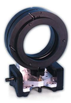
OMS 160 is an optical mount for non-standard optical lens with outer diameter of 160 mm featuring similar mechanical design as OMS 120. It has a 4-axis movement capability: 2 linear displacements (x, y directions) and 2 independent angular positioning. The system can be mounted on a standard optical rail or table. The mount is fabricated from aluminium and murytal.
